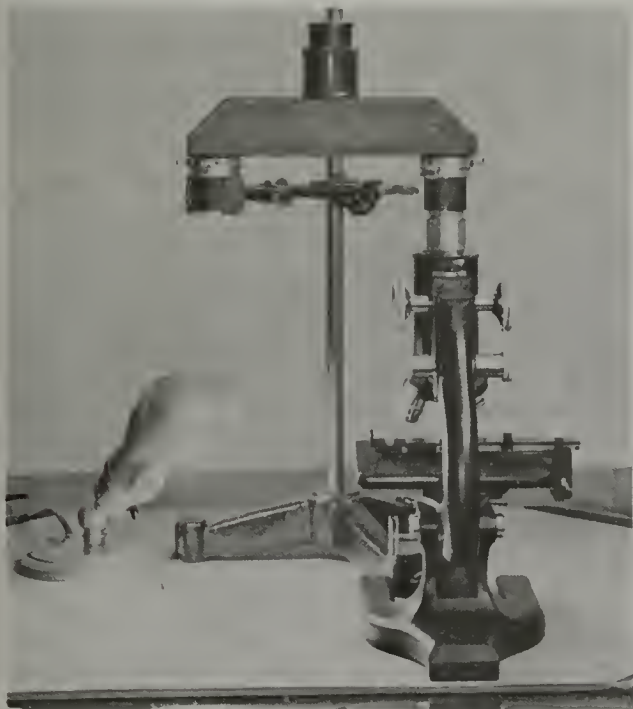
FIGURE 9. Microscope and comparison ocular. The Munsell charts are placed on the table under the open end of the ocular.
